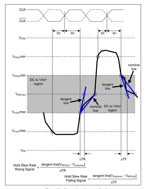
Figure 23 - Illustration of tangent line for tIH
