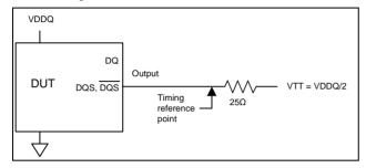
Figure 16 - AC timing reference load
