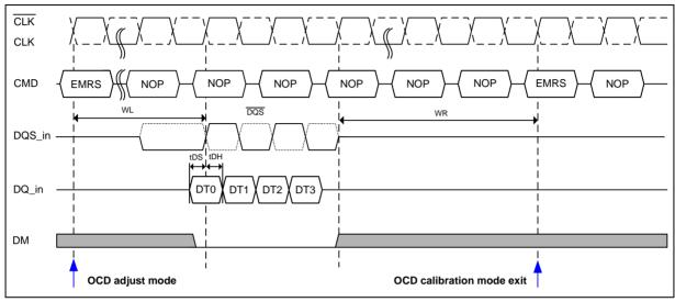
Figure 7 - OCD Adjust Mode
