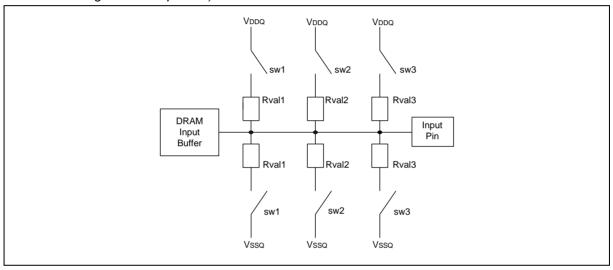
Switch (sw1, sw2, sw3) is enabled by ODT pin.
