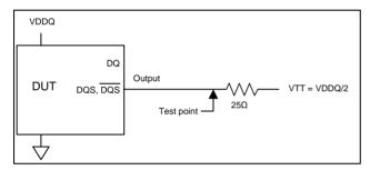
Output slew rate test load
