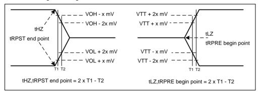
Figure 18 - Method for calculating transitions and endpoints
