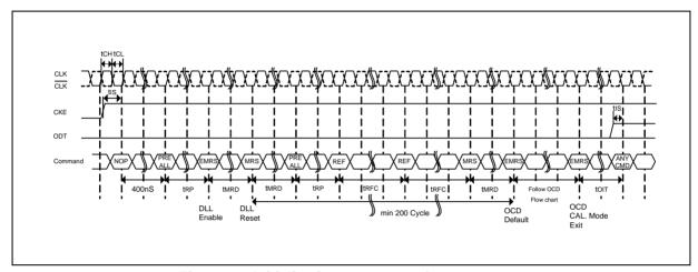
Figure 1 - Initialization sequence after power-up
